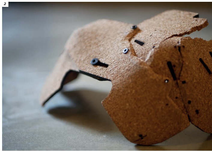
▲ Welded Chassis, and Laser Cut shells Initially designed as a ruler to latch onto rock surfaces, the chassis evolved during site exploration. Adjustable laser-cut cork pieces were developed to wrap around the welded steel frame, exploring how an architecture might adapt and latch onto its habitat.
