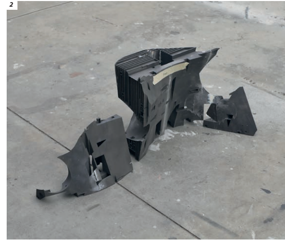
▲ Unfinished Fragment Development A model fragment for The Line in its unfinished state, 3D printed in nylon and joined with epoxy.
