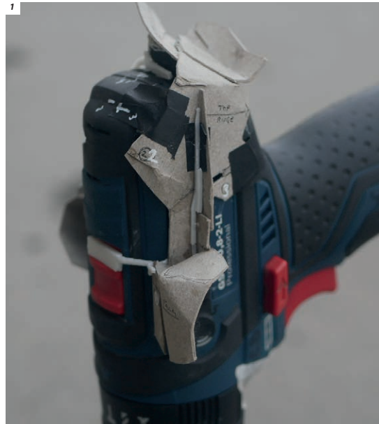
▲ A Drill Jacket Augmenting a slightly broken drill to become operational again by wearing a jacket that forced the hand into the correct position. Hand cut cardstock during lockdown, with no access to a workshop.
